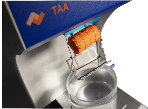
Fig 1 : TAA The basket is dropped horizontally to a height of (25 \pm 5) mm above the surface of the water
