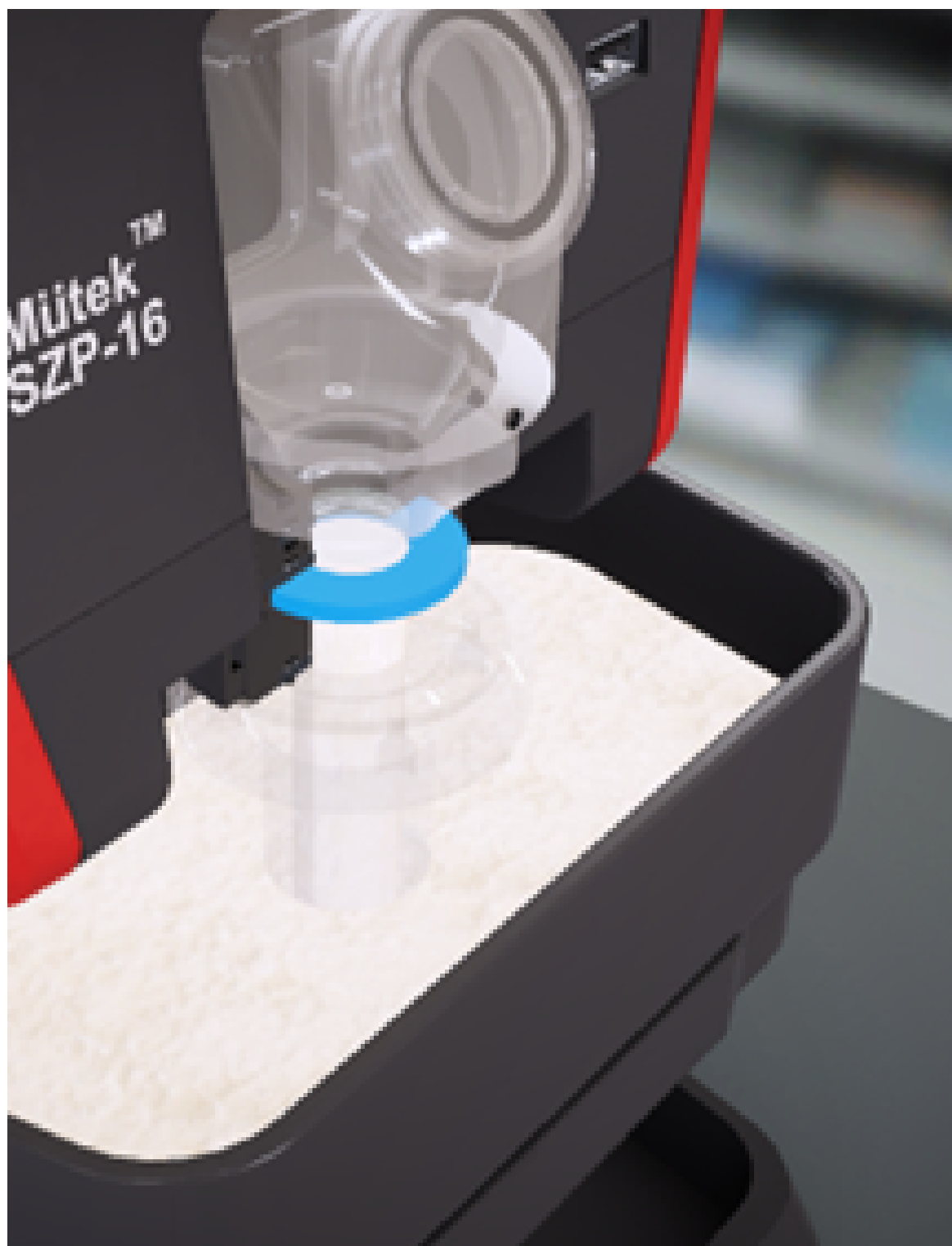
Figure 2: Measuring cell cut view SZP-16 with sample
